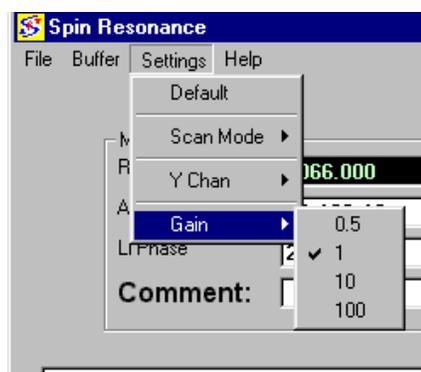
“Gain” menu item, currently chosen gain will be checked in the menu. The setting of the gain for every channel is not affected by the switching of channels. The default settings (gain=1 for all channels) are restored at the next start-up of the software.
