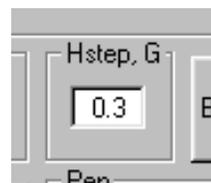
**NOTICE:** Although the value of the step is not limited, please keep in mind that the maximal number of points, which can be memorized by the software, is  $N_{MAX}=10000$ . Thus, the value of sweep diapason divided by the step value ( $N=sweep/step$ ) should not exceed this number. Besides that, the precision of AD converter - sweep generator system
