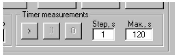
**IMPORTANT:** Previously mentioned limitations on the total number of measured points still apply here, thus ratio of interval/step should be less than 10000. Depending on specifications of the PC used, reliable minimal time step interval will be also limited. For detection safety it is not recommended to use step value  $<0.05\text{sec}$ .
