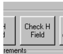
button causes the message to appear, which compares actual H field (measured by gaussmeter) to the one calculated using the recent setting constants. The acceptable difference between the two values should not exceed 0.1% of the sweep range.
