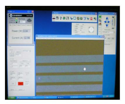
$\lambda_{LAS}$ = 532 nm Laser power ~ 400 mW Focal distance : 12-15 mm Scanning speed: 0.3 mm/sec Process rate: 5×10<sup>-3</sup> mm<sup>2</sup>/sec
